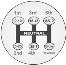
The more relaxed your hand is, the easier it will be to make your gear changes. Avoid 'gripping' the gear lever tightly. The speeds shown on this diagram are approximate and may vary from car to car
